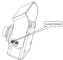
3. Clean the installation area and attach the camera as below.
