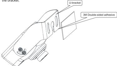
2. Loosen the screws to the U-bracket.
