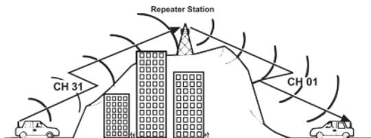
Operation with the aid of a Repeater Repeater Station (Duplex).
