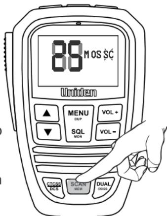
Press **[SCAN]** and scanning of the current memory group will start. **SC** flashes during scan.
